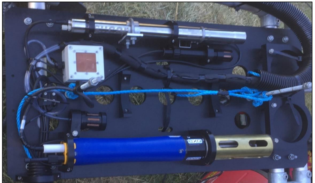
Figure 8: An example set up for the LOCATE sensor pod components. The submersible sensors pictured consist of the Xylem EXO2 multi-parameter sonde, an S::Can Spectro::lyser and a Vaisala CO2 sensor. The atmospheric sensors (not pictured) consist of a Vaisala met station and a Skue Instruments PAR sensor.
