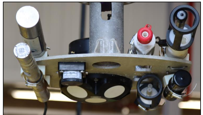
Figure 11: The C-worker 4's Oceanographic Payload suspended from under the surface vehicle.
